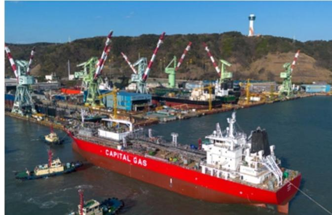
US-listed **Capital Clean Energy Carriers** ordered four ammonia-ready LCO<sub>2</sub> low-pressure (LP) LCO<sub>2</sub> carriers in **July 2023**, to be built at **HD Korea Shipbuilding & Offshore Engineering's** (HD KSOE) **HD Hyundai Mipo**, all classed by LR. The LP LCO<sub>2</sub> carriers are designed to operate at ~ 8barg and -55 °C.
