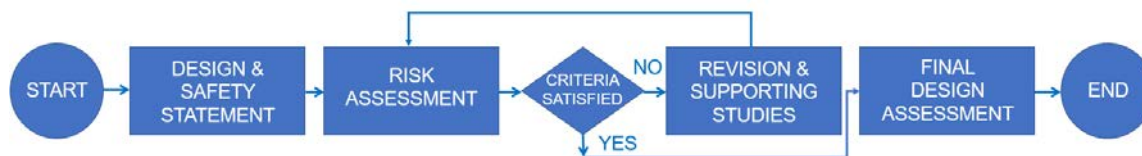
Figure 3 Process for Risk Based Design (15)
